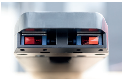
Safe load pick-up thanks to integrated sensors in the fork tip
