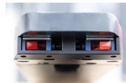
Safe load pick-up thanks to distance sensors in the fork tip.
