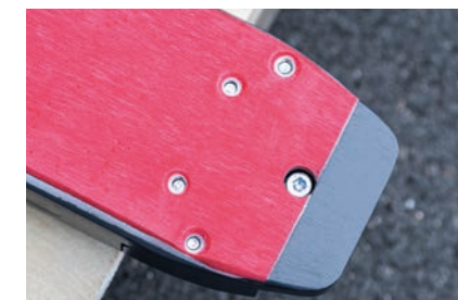
AGV sensor fork with obstacle detection in the tip and anti-slip coating.
